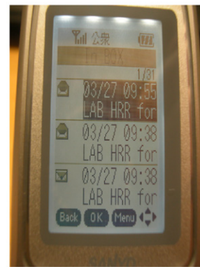
Fig. 3. Sample HRRS subsystem alert message sent via e-mail and cellular phone.
